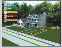
You may not use any mechanical device (backhoe, trencher, auger machines, rototillers, etc.) to dig within 18 inches of either side of the marks left by the utility companies.
